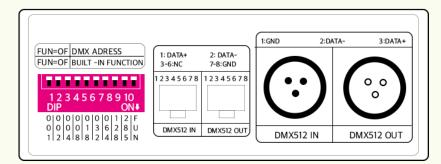
DMX signals can be received when coding switch FUN (10) is switched OFF. When coding switch FUN (10) is ON, the other functions are:
